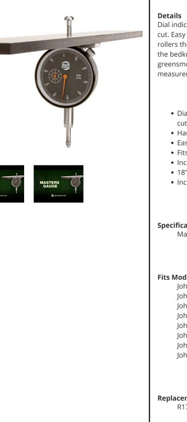
Dial indicator accurately measures desired height of cut. Easy to use. Place the bar on front and rear rollers then push the measuring rod until it touches the bedknife edge. Hard anodized aluminum. Fits all greensmowers. Easy to read dial indicator. Displays measurements in .001" increments. 18" length.
